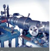
The diaphragmless shock tube for the study of high-speed flows. KB series valves provide experiments with high productivity and repeatability.
