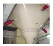
Vibrating bottom eliminate hang-up of loose material at the bottom of a hopper mainly while hang-up on vertical walls still exist.
